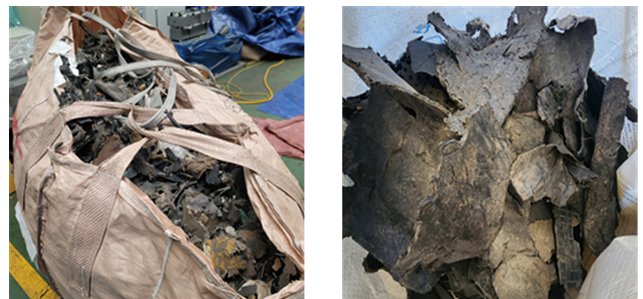
Figure 1. Pictures of raw ASR fluff (left) and sorted HCPP from ASR (right).
